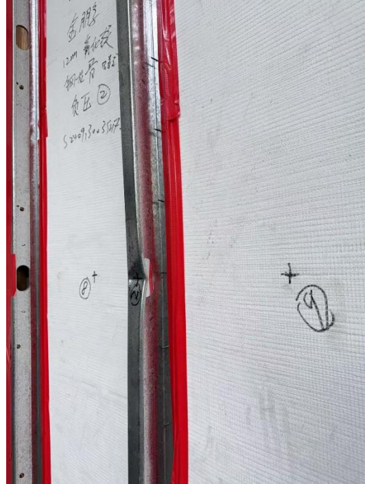
Transfer Load Test Failure- Negative Specimen
