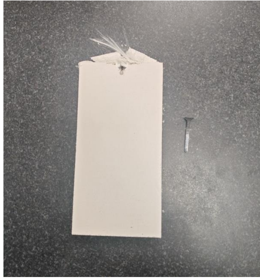
Fastener Lateral Load Test Failure- Dry specimen
