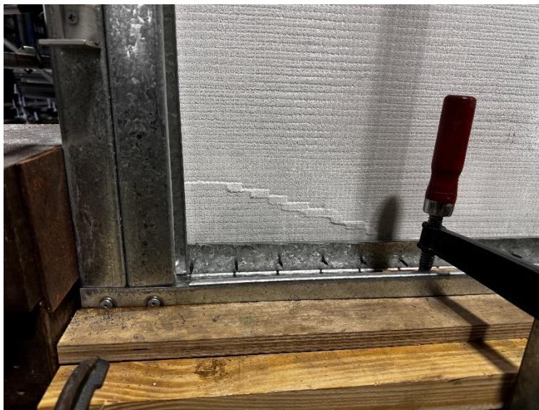
Racking Shear Test Failure – Wet Specimen
