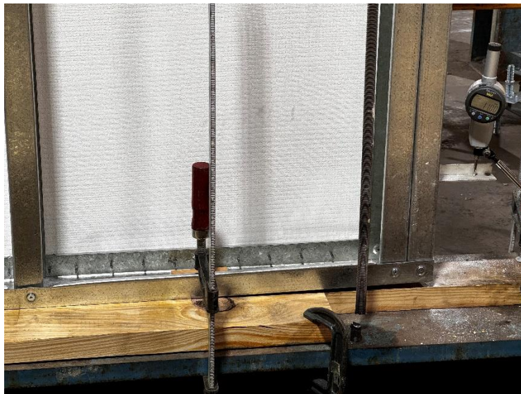
Racking Shear Test Failure – Dry Specimen
